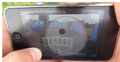
Figure 1. CODA display integrated in MAV-VUE interface, for use in navigating in an outdoor environment.
