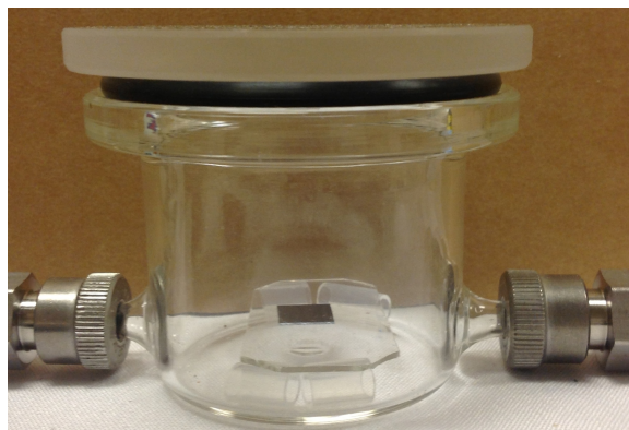
Figure 2-13: The flow controlled solvent vapor annealing chamber.
