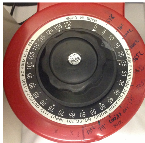
Figure 2-17: A variable voltage regulator was used to alter the AC voltage applied to the heating element.
