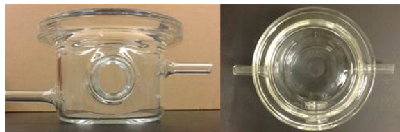
Figure 2-15: The glass chamber used for solvothermal annealing.
