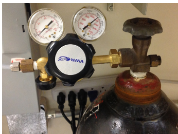
Figure 2-3: N_2 was used as the carrier gas for the flow controlled solvent vapor annealing setup.
