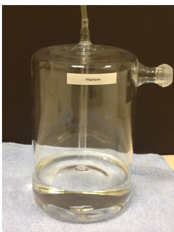
Figure 2-8: A glass chamber was used to contain the solvents. These pieces were custom-made.
