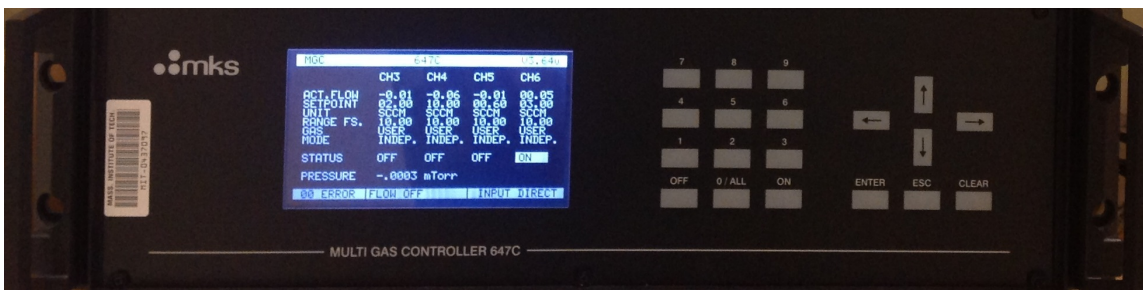
Figure 2-6: The control box for the flow controllers which is capable of operating eight channels simultaneously.
