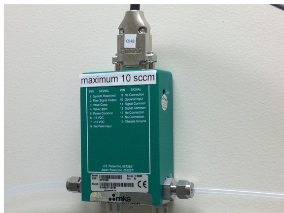
Figure 2-5: Mass flow controllers were used to regulate the mass/volumetric flow rate of the carrier gas before it was sent to the solvent sources.
