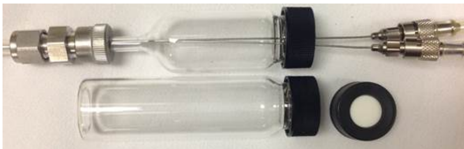
Figure 2-12: A modified glass vial was used with a septum top to facilitate the mixing of multiple solvent streams.
