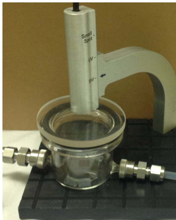
Figure 2-14: The solvent vapor annealing chamber underneath the spectral reflectometer which allowed for in situ film thickness measurements.
