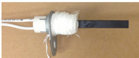
Figure 2-16: A silicon nitride hot surface igniter was used as the heating source for the solvothermal annealing.
