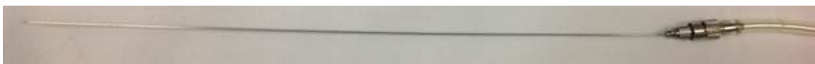
Figure 2-11: A diameter reduction of the saturated solvent vapor line was completed by using a 0.6 mm ID needle.
