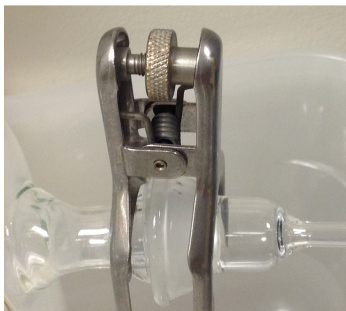
Figure 2-9: The ball and socket connection on the solvent container.
