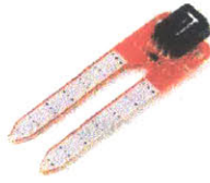
Two wire resistive sensor - excludes microcontroller - equivalent to home made solution ~$10
