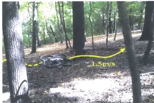
Figure 42 – UAS Navigation through Learned Monocular Reactive Control
