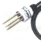
Time domain impedance dielectric reflectometry Probe ($1000 - $2000)
