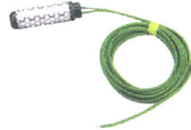
Gypsum block resistive Moisture Sensor (~$50)
