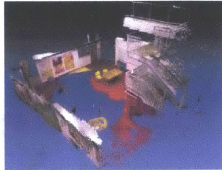
3D reconstruction of local environment using Kinect Sensor
