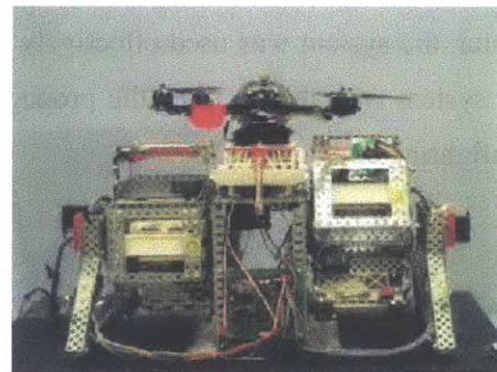
Figure 47 - Autonomous Battery Swap and Recharge Station
