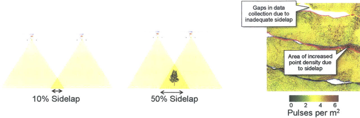
Figure 68 – Illustration of Sidelap and Impact on Data Collection
