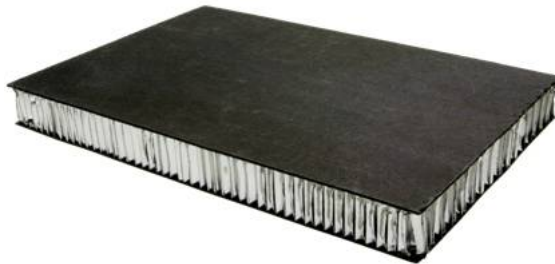
Figure 1: Example of honeycomb sandwich composite used commonly in aerospace structures [2].
