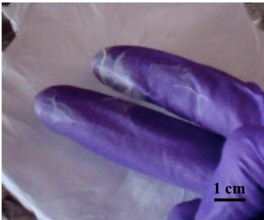
Figure 3-1. Optical photograph of loose fibers being removed from the surface of an electrospun fiber mat due to gentle contact with a nitrile glove. Scale bar for this image is 1 cm.
