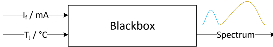
Figure 6.4 - A multi-input multi-output subsystem model for optical transient LED models
