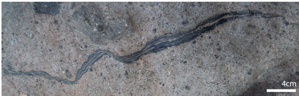
Figure 5-1. Field photo of the shear band. Aphanitic pseudotachylyte layers of the shear band are interspersed with cataclastic layers. Photograph illustrates the lateral variation in thickness and its morphology, which suggests formation in viscous magma in the conduit.
