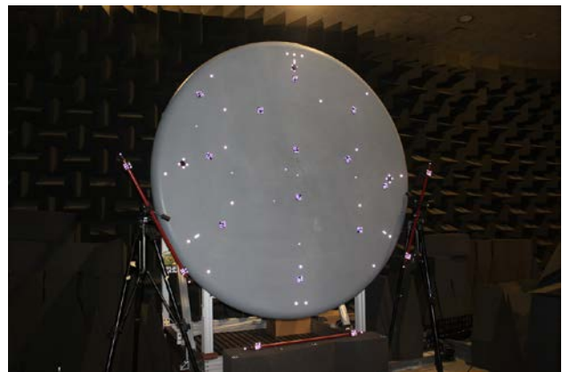
Figure 4. Set up for the coordination of the targets on the surface of the microphone array disk.
