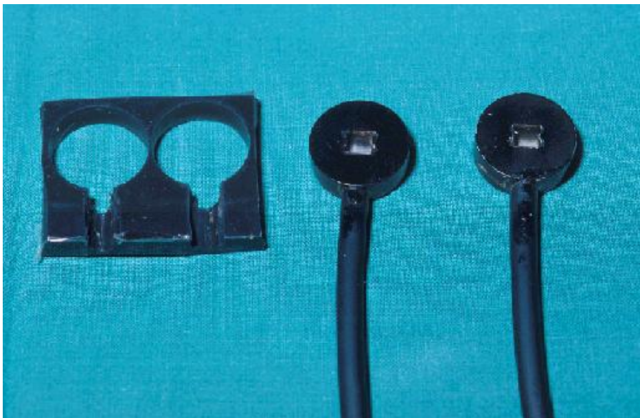
Figure 4.4: Near infrared spectrometer probes and a rubber optode holder (NIRO 500, Hamamatsu Photonics KK, Hamamatsu, Japan)
