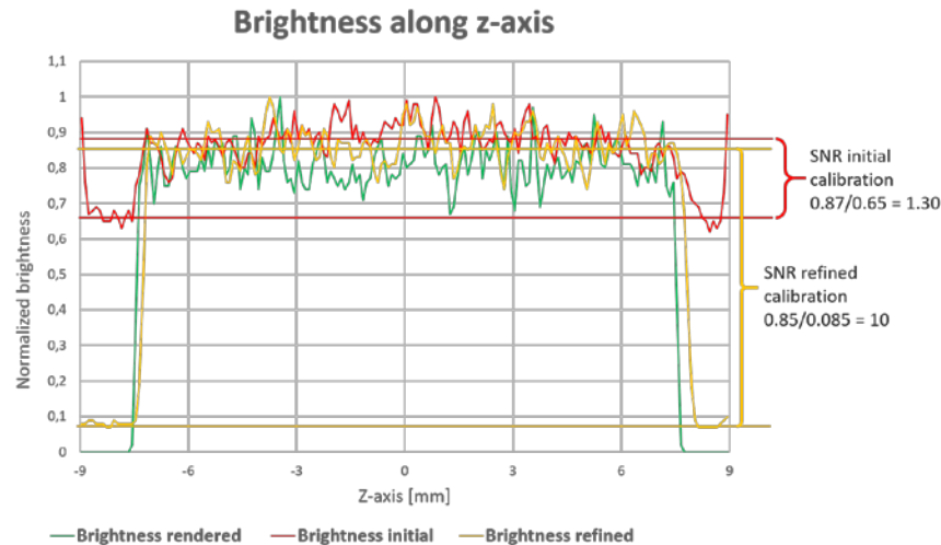
Fig. 10: Z-axis intensities of the reconstructed voxel spaces indicates the large improvement in ghost level intensities between the reconstructions with the outdated initial- (red line) and the reconstruction using the refined calibration (yellow line).
