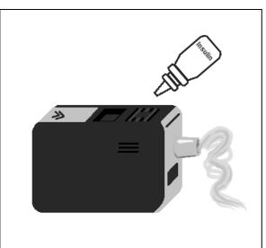
Figure 4: Simplified image of the Dance-501 device along with a separate insulin container. This device uses a vibrating mesh micropump technology developed by Aerogen; figure adapted from [50].
