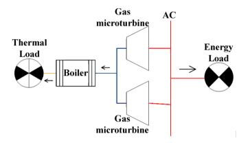
Figure 1. CHP system scheme
