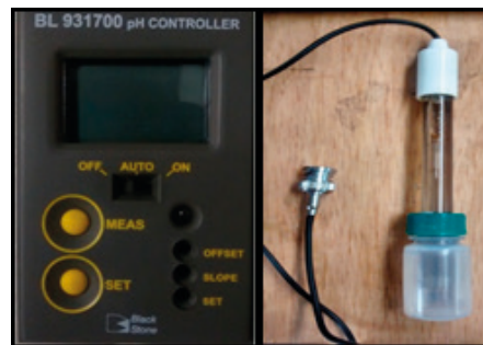
Fig. 5. Installed pH. indicator controller. Source: Authors
