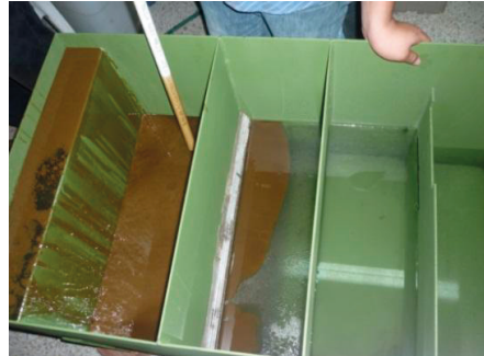
Fig 1. CPI Separator equipment. Source: Authors
