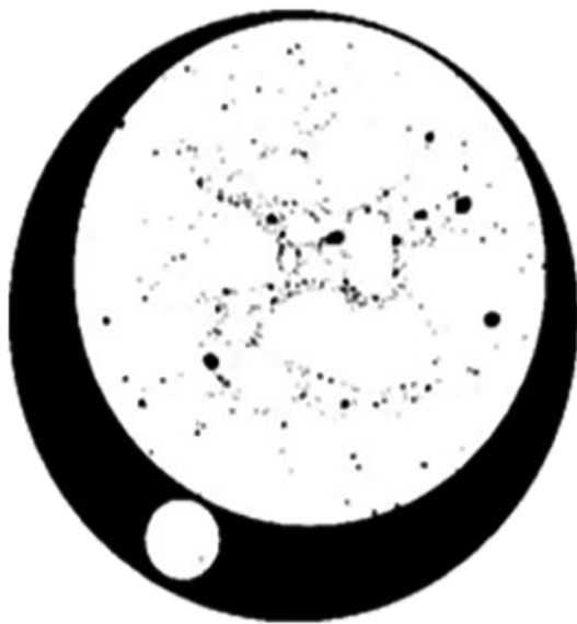
FIGURE 8 Identification of voids contained by each composition
