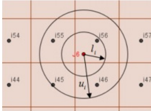
Fig. 1. Coverage concept according to Berman's model.
