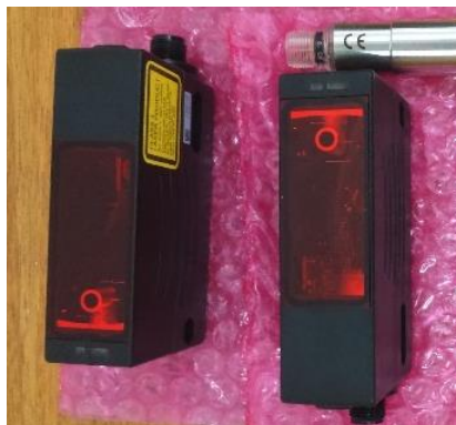
Figura 18 Sensor laser 45 LMS de Rockwell Automation.
