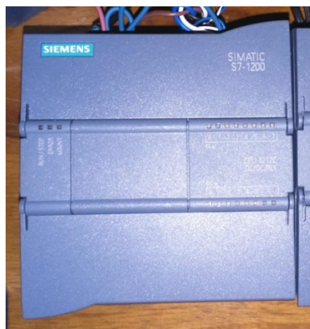
Figura 27 PLC S7 1200, CPU 1212C
