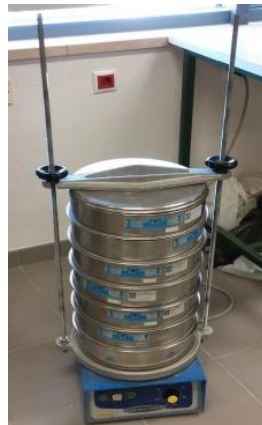
Figure 3.3: Mechanical sieving of sand.
