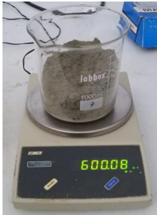
(a) Weigh of cement
