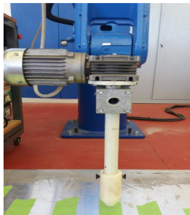
e) Single fuse extruder with nozzle
