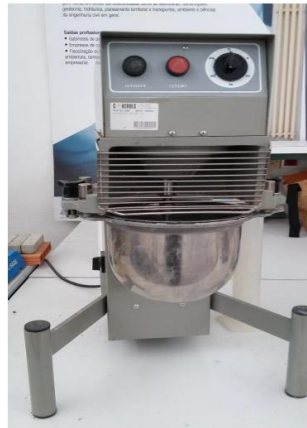
(b) Mixing of mortar
