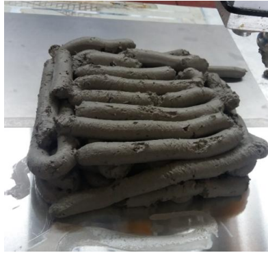
a) Mix M15 printed with pipe
