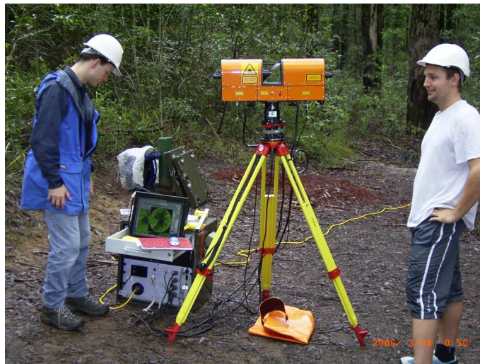
Figure 15: Photograph of the Echidna laser scanner in Northumberland national forest near Sydney. Dr. Darius Culvenor is in the left and Dr. Nicholas Goodwin on the right. Photograph by Professor Jan-Peter Muller.
