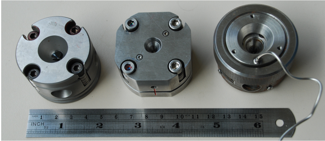
FIG. 2: A photograph of various diamond anvil cell devices used in this work. (left) The cell is referred to as a Mao symmetrical cell which consists of a four-screw piston-cylinder set-up. (middle) This cell is of a similar set-up to the Mao cell and is designed and built by EasyLab Technologies Ltd, UK. (right) A membrane cell (EasyLab Technologies Ltd, UK) in which pressure is generated by pumping gas in an expandable membrane which pushes the piston half of the cell into the cylinder half.
