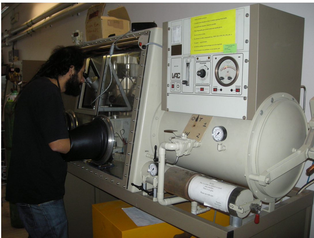
FIG. 6: A photograph of a glove box at UCL, designed and modified specifically for diamond anvil cell loadings.
