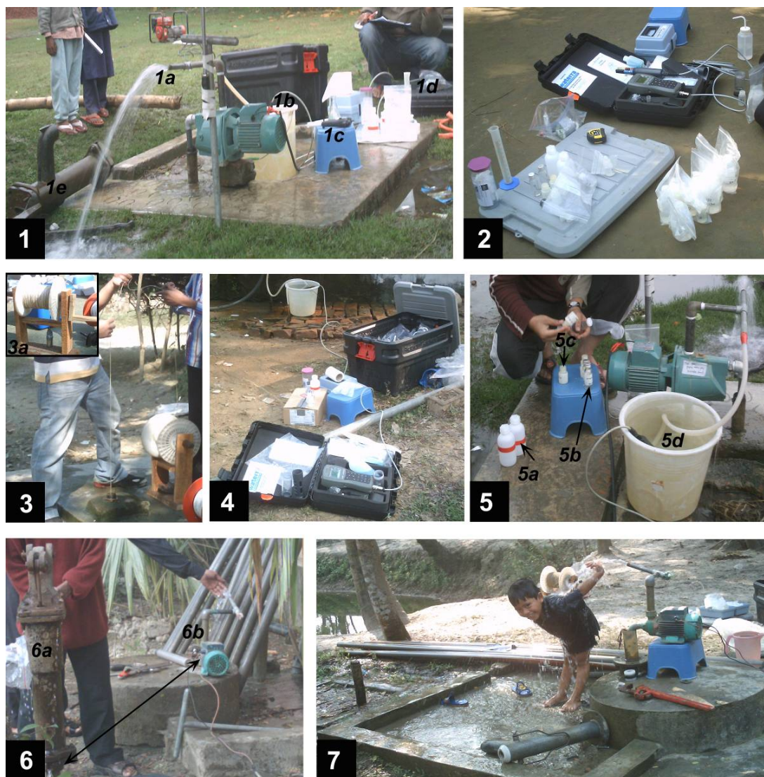
Figure 5-4: Photographs showing field-camp activities during the groundwater sample collection in December 2007 to February 2008 in Bangladesh. 1. Total activities at a sampling site: 1a well purging, 1b flow-cell, 1c onsite titration for \text{HCO}_3^- measurement, 1d onsite measurement of field parameters; 2. Onsite calibration of the Multiparametre instrument; 3. Well-depth measurement using self-designed (3a) 400 m string in a spool with number marking (every 5 metres) and a weight at the end; 4. Flow-cell and multiparametre instrument are in use; 5. Sampling: 5a radiocarbon sample bottles, 5b stable isotope sample bottles, 5c sample bottles for major ions and trace-element analysis, 5d flow-cell (inside the bucket) kept submerged; 6. Wells were sampled: 6a shallow well, 6b deep well, are within 2 m distance; 7. Well-purging before setting up flow-cell.
