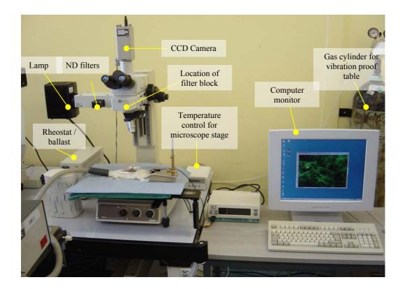
Figure 2.5 The complete intravital microscopy setup.
