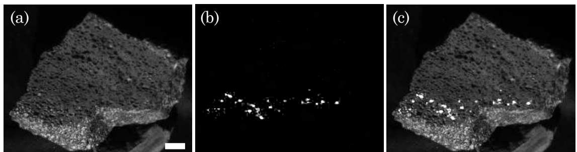
Figure 6.20. Magnified Foculus captured image of KV007 epifluorescence at a distance of 2m through the green filter. a) with Solex illumination; b) with 375nm laser illumination and 150s total exposure; c) images 'a' and 'b' combined to show the position of the fluorescence within the lava vesicles. Scale bar 1cm.
