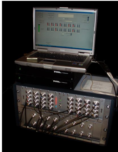
Figure 3.2: UCL topography system with 32 laser sources and 16 detectors.
