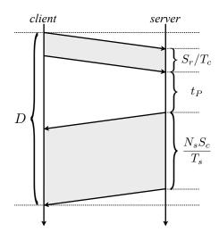
$D = t_{RTT} + \frac{S_r}{T_c} + t_P + \frac{N_s S_c}{T_s}$ (6.7)
