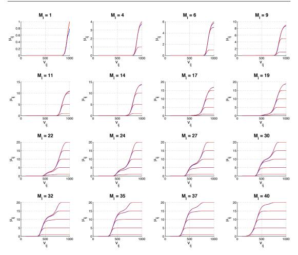
Figure 5.4: Expected number of won bids  $\mathbb{E}[X^{ij}]$ . Blue curves correspond to experimental simulation, red curves to (5.6). Each curve corresponds to a different  $m_{ji} \in \{1, 5, 10, 15, 20\}$ . All curves are present in all graphs, but overlap in the cases where  $m_{ji} > M_i$  since the number of won items is clamped at  $M_i$  in that case.
