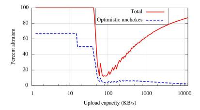
Figure 2.1: Expected percentage of upload capacity not resulting in direct reciprocation (figure taken from [254]).
