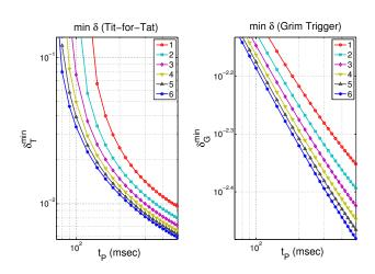
Figure 6.6:  $\delta_T^{\min}$  and  $\delta_G^{\min}$  for the simulation run of Table 6.4 (the legend in both graphs shows different values of  $N_s$ , the number of clients that the server is serving simultaneously).
