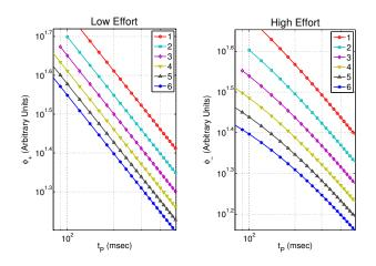
Figure 6.5:  $\phi_+$  and  $\phi_-$  for the simulation run of Table 6.4 (the legend in both graphs shows different values of  $N_s$ , the number of clients that the server is serving simultaneously).
