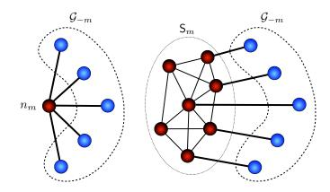
Figure 3.1: A malicious node  $n_m$  and its sybil strategy  $S_m$ . The links between  $n_m$  (or  $S_m$ ) and the rest of the network,  $\mathcal{G}_{-m}$ , are the *attack links*.
