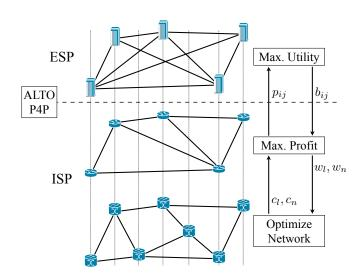
Figure 7.1: ALTO/P4P and an interface between overlay-based Edge Service Providers and ISPs.
