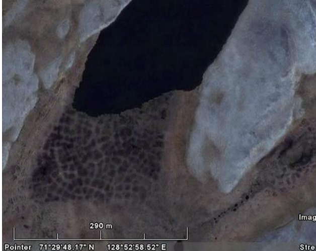
Figure 2.11. Polygonal patterned ground at lake LS-7 in the Lena delta (GoogleEarth™ image, accessed 14.09.2008).
