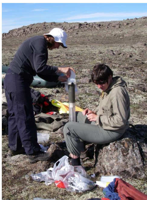
Figure 3.1. Extruding HON-Kajak core from lake PTHE (left – right V. Jones and N. Solovieva)
