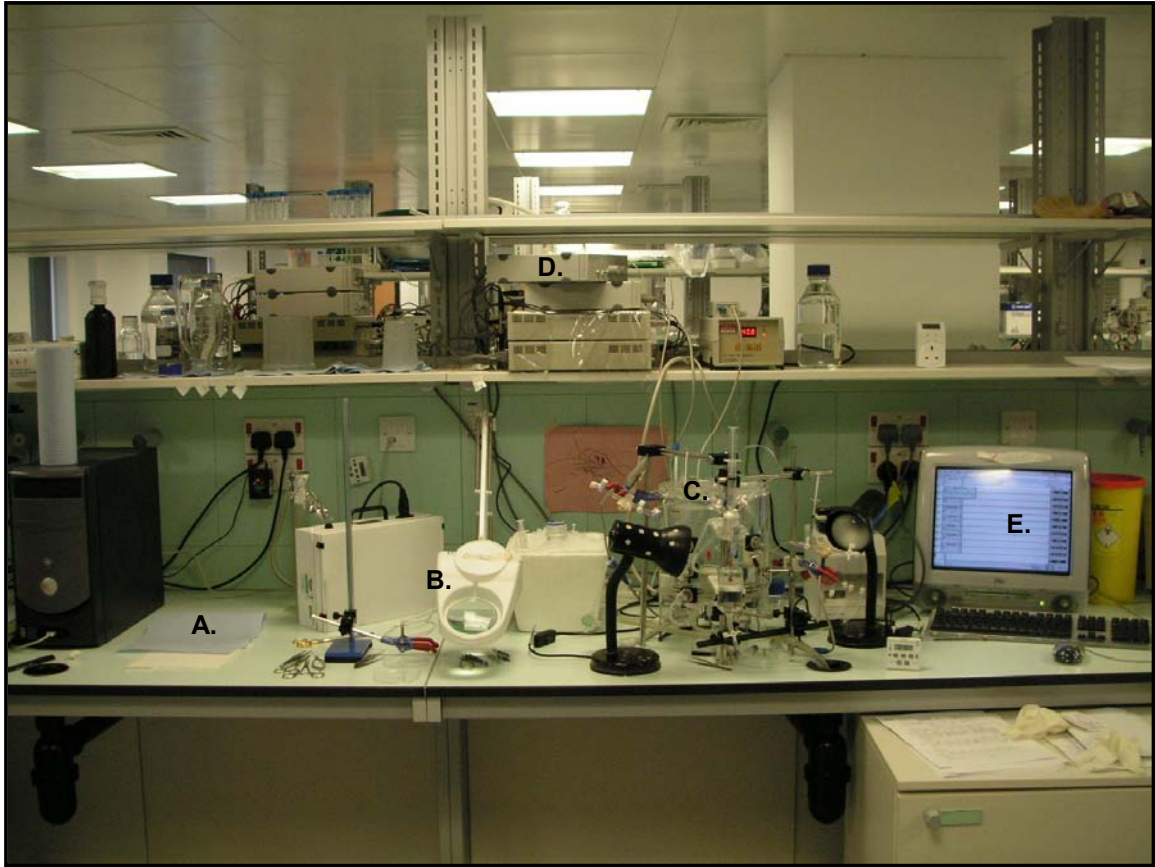
Figure 2.2: The perfusion system used for studying isolated mouse hearts: A) dissection area, B) cannulation area, C) perfusion apparatus, D) PowerLab electronics and E) computer used for data acquisition.
