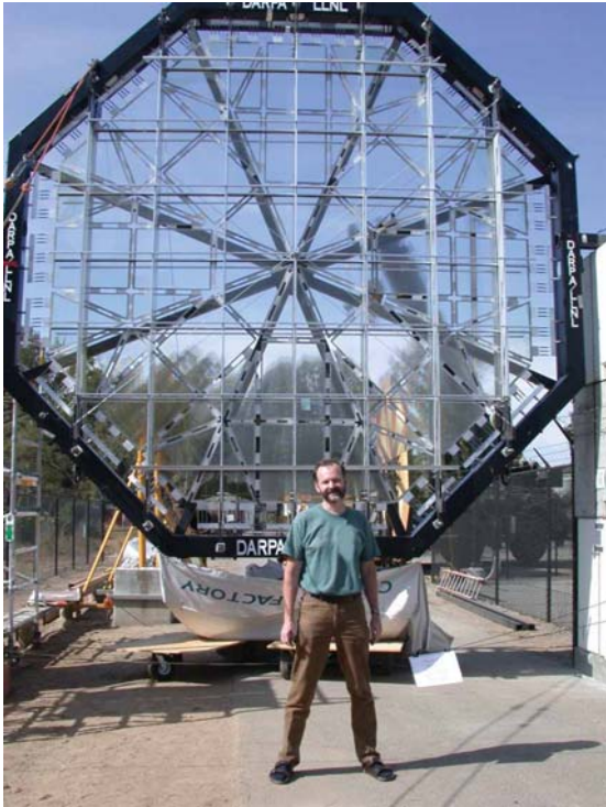
Figure 15 : Robert Lang with the 5m Fresnel foldable lens designed using an algorithmic application of graph theory.
