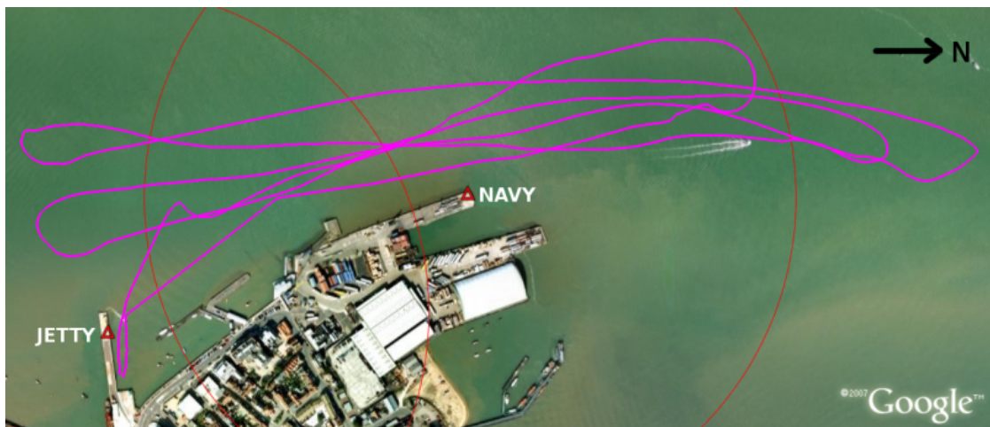
Figure 6.5: Plot of THV Alert 's course, showing total station locations with 400 m range circles
