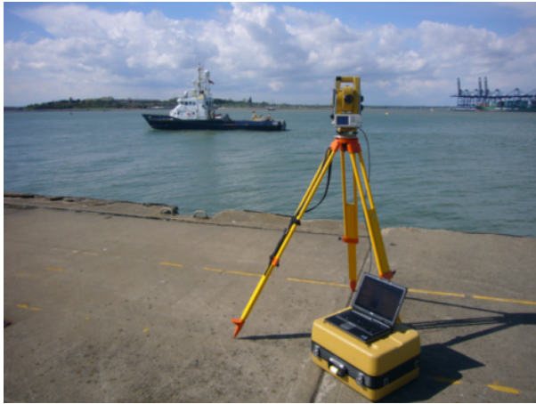
(a) Total station tracking THV Alert
