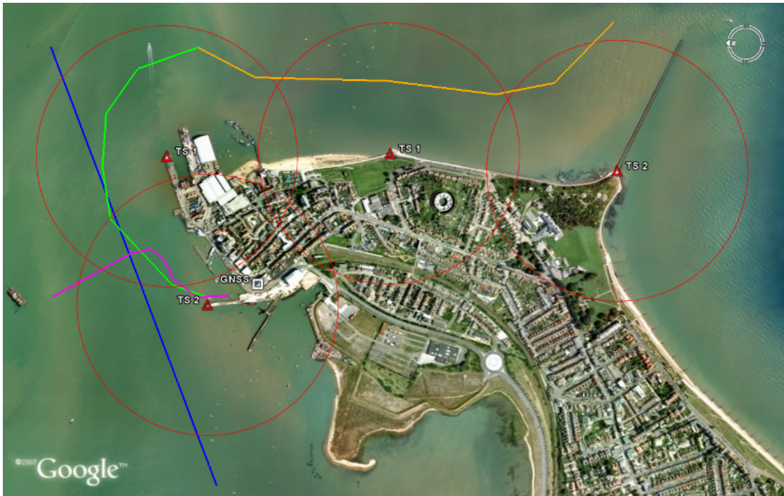
Figure 6.3: Initial design of Harwich data collection exercise, showing Alert's course and total station locations with 400 m range circles
