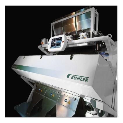
Figure 5.2: The three chute monochromatic Buhler Sortex Z+ sorting machine. Picture ©copyright Buhler Sortex Ltd, 2008. Reprinted with permission.
