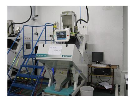
Figure 5.20: Buhler Sortex Z1 sorting machine and PC based capture system. Picture ©copyright Buhler Sortex Ltd, 2008. Printed with permission.
