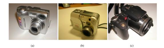
Figure 4.6: The three different cameras used to acquire the colour variation database. These are 4.6(a): a Nikon Coolpix 4600, 4.6(b): an Olympus Camedia C40 Zoom and 4.6(c): a FujiFilm FinePix 6900 Zoom.
