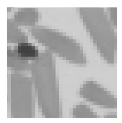
Figure 5.5: A portion of the capture stream that clearly shows the individual grey-levels that are recorded over a small spatial region and short time frame. Rows in the image are grey level values captured over time, columns indicate spatial position across the chute. Picture ©copyright Buhler Sortex Ltd, 2008.
