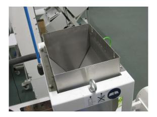
Figure 5.24: Top chute to be filled with rice on the Buhler Sortex Z1. Picture ©copyright Buhler Sortex Ltd, 2008. Printed with permission.
