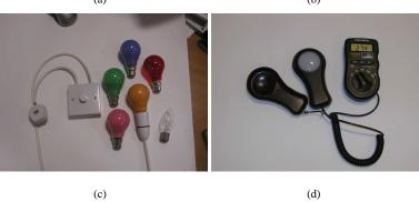
Figure 4.5: Locations and equipment used to create different lighting conditions. 4.5(a) shows the naturally lit lounge and 4.5(b) shows the office lit by florescent bulbs. 4.5(c) shows the bulbs and dimmer switch used create local lighting variation, 4.5(d) shows the light meter used to approximately monitor the ambient lighting conditions.
