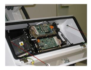
Figure 5.23: Camera and sorting electronics. Picture ©copyright Buhler Sortex Ltd, 2008. Printed with permission.
