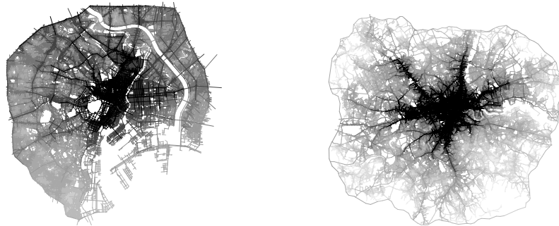
Figures 4 and 5 showing least angle integration (normalised closeness) for metropolitan Tokyo (left) and London within the M25 (right) in each case showing a variant of the 'deformed wheel' structure, with multiple rims in the case of Tokyo
