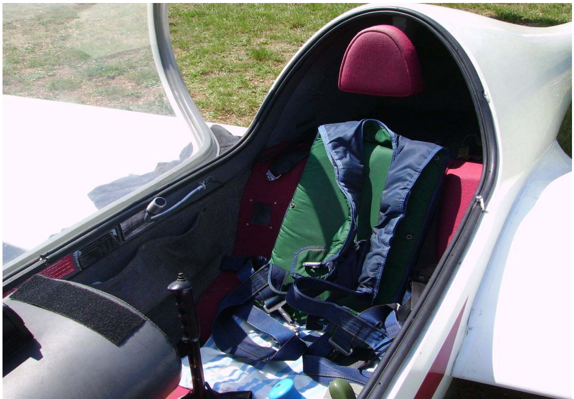
Back seat with parachute. In the foreground are the stick and the airbrakes and trim levers.
