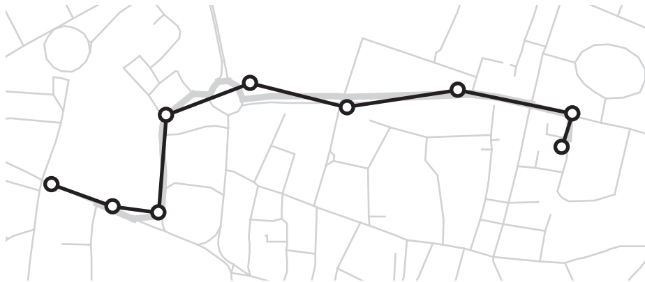
Fig. 2. Sample GPS trace (black) and the path as attached to the topological base map data (thick gray). This example uses OpenStreetMap data rather than the OS ITN layer used for the actual experiments.
