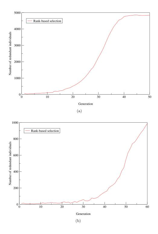
Figure 5.12: Redundancy of individuals in a GA run using Rank-based selection with (a) 5000 individuals and  $\mu$ =0.0001 (b) 1000 individuals and  $\mu$ =0.001.
