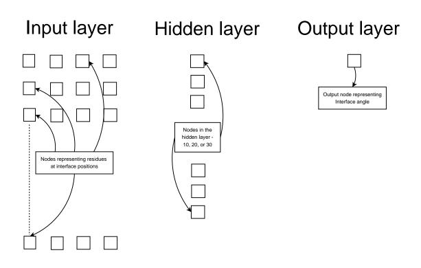
Figure 5.9: Architecture of a fully connected network. Not shown in the figure are the connections between every pair of nodes in the input layer and hidden layer and between nodes in the hidden and output layer.
