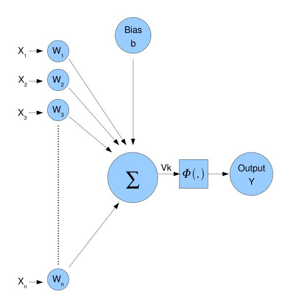
Figure 2.1: Schematic representation of a neurode in an artificial neural network. Figure shows the inputs to the neurode X1, X2, X3...Xn, weights of synapses W1, W2, W3...Wn, summation function  $\sigma$ , bias b, activation function  $\phi$  and output Y.
