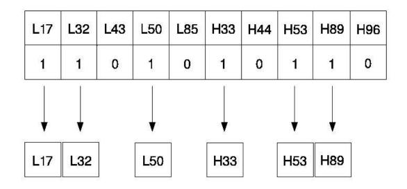
Figure 5.10: An individual to represent 10 interface positions. From the string shown, those *alleles* with a 1 imply the inclusion of the residue at the respective interface position for training and validation of the neural network.
