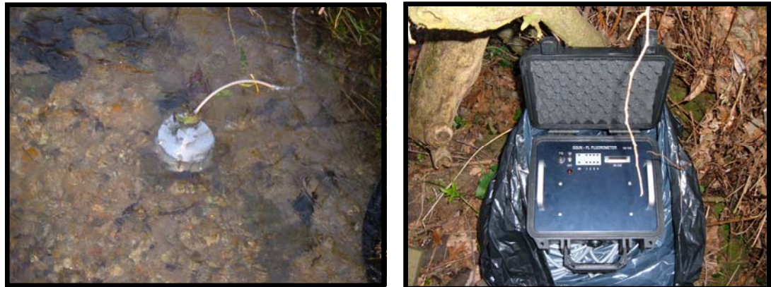
Figure 4.7: Field Fluorometer (left) and datalogger (right); from Neuchatel University
