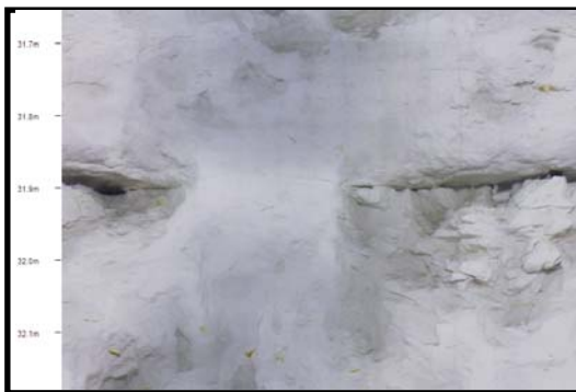
(c) Solutionally enlarged fracture up to 2 cm high at 78.6 m AOD
