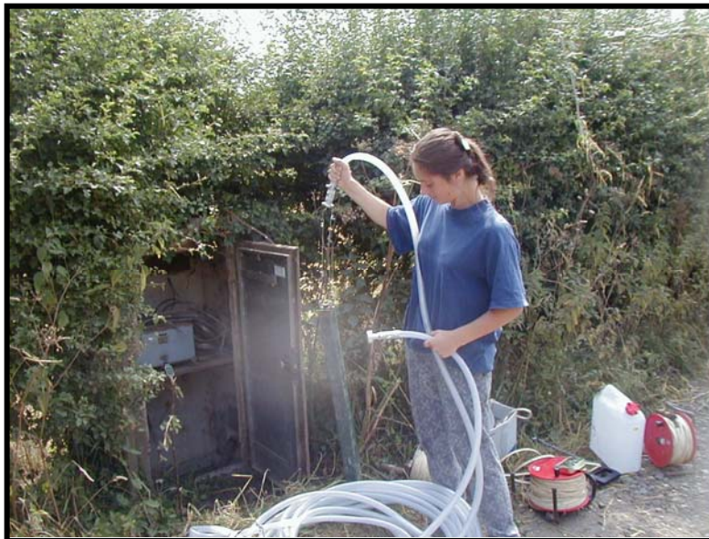
Figure 6.2: Hosepipe and weight at Peasmore Borehole (SU 47/121)
