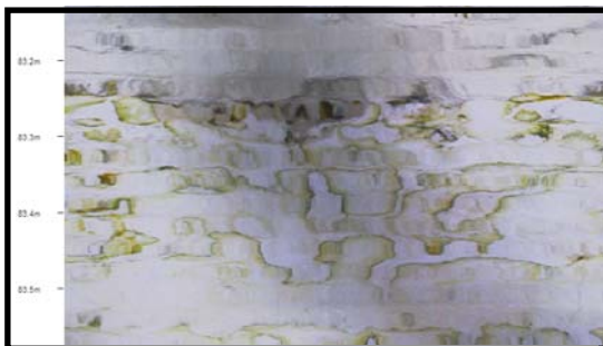
(e) Conduits, aperture ~ 1 cm at 27.2 m AOD on a hardground
