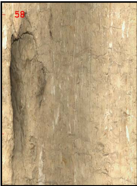
(c) Vertical fracture at 90.7 to 91.4 m AOD (58 to 58.6 m below datum)
