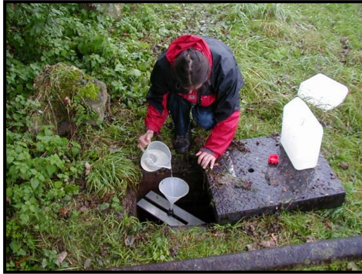
Figure 6.3: SBDT tracer injection system, Grumble Bottom Borehole (SU58/101). Top of hosepipe is resting on a metal plate that spans the top of the borehole casing (photo Alex Gallagher).
