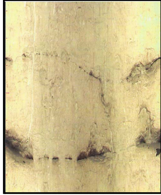
(b) Fractures with multiple openings at 86 and 85.7 m AOD
