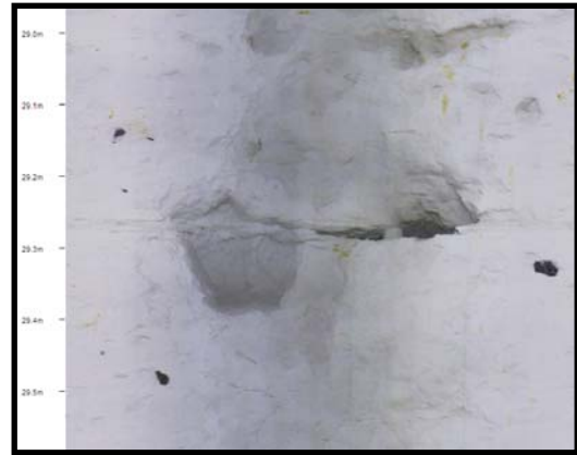
(b) Solutionally enlarged fracture, up to 3cm high at 81.3 m AOD
