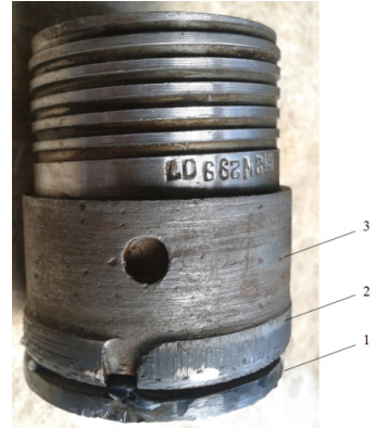
Fig. 2. Thermomechanical drill bit: 1 – friction plate; 2 – matrix; 3 – drill bit body.
