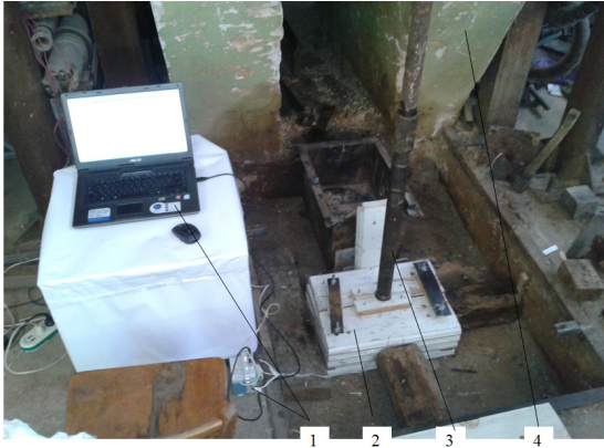
Fig. 1. General view of the stand: 1 – measuring and computing complex; 2 – the model of absorbing horizon with spacers; 3 – a string of drill pipes; 4 – base of the drilling rig.
