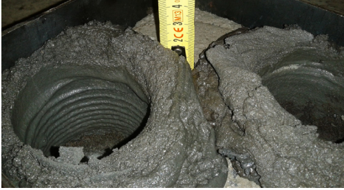
Fig. 4. The view of the melt (plaster stone) obtained at a rotation frequency of 500 \text{ min}^{-1} and an axial load equal to 700 \text{ daN} , for TPCM with a component ratio of 1:3.
