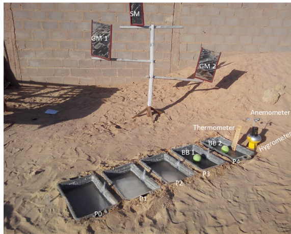
Figure 4. Photograph of the experimental brine pans on Chott Merouane-El Oued
