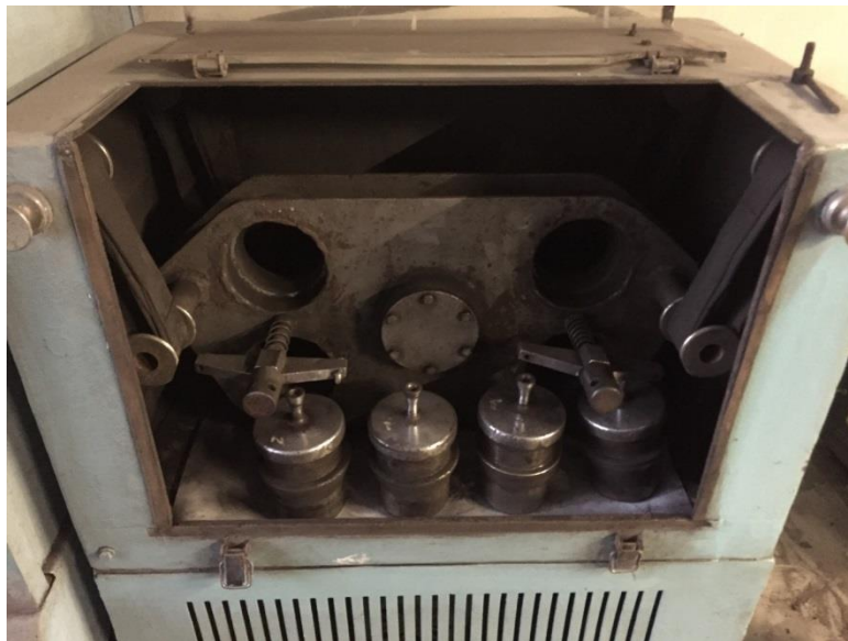
Fig. 8. Diagrams of the movements of the grinding media in a cylindrical mill. A) Simplified model of the gearing; B) \omega_1, \omega_2 , pulsations (angular speed) for jar and cylinder; C) image of the grinder. The rotation center of the jar, C_j , is at once his eccentric relative to the rotation center of the system, C_e .
