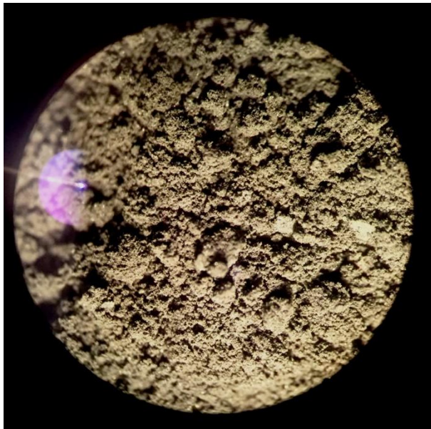
Fig. 10d Glass fibers and metals in the class -0.05 mm after screening
