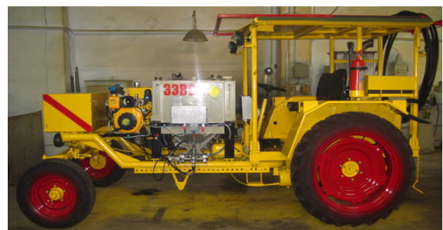
Figure 4. Self-propelled (blasthole) charger for EEs of ZEVS-type (general view)
