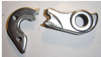
Fig. 1 - Typical expected failure of the lever
