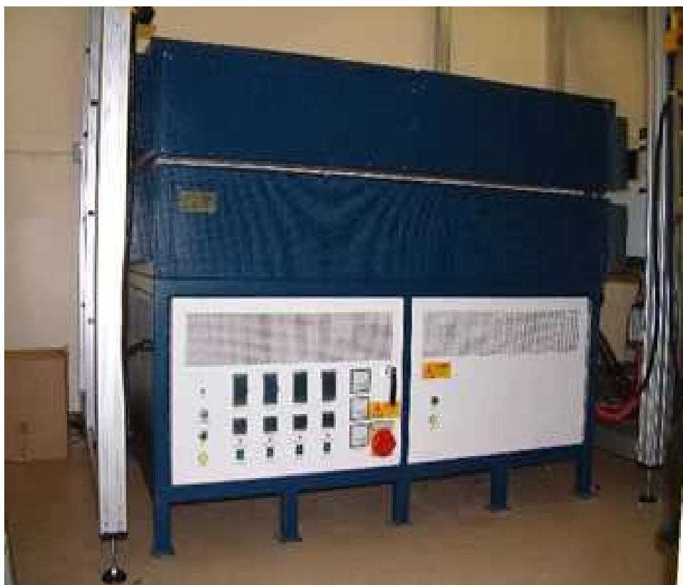
Figure 2.5: The LUSI furnace, consisting of four temperature-independent bays and computer controlled temperature profile. The ink-jet printer and X-Y measurement stage are to the right hand side of the furnace.
