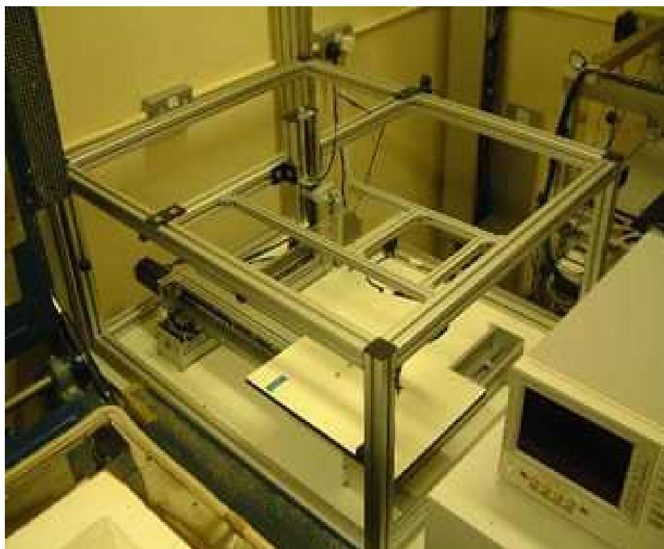
Figure 2.6: LUSI features an X-Y measurement table permitting high throughput analysis. The table measures 500 \times 600 mm and is precise to 1 \mu\text{m} , subject to temperature fluctuation. A hot plate is mounted on the table and is independently controlled up to 250^\circ\text{C} .
