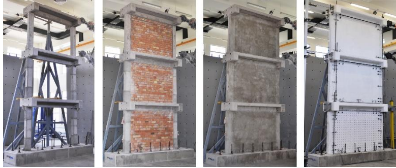
Figure 13. Retrofitted model tested at the University of Patras
