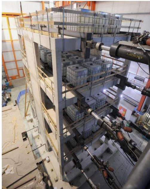
Figure 11. Building with RC infilled bay tested at the ELSA lab in JRC
