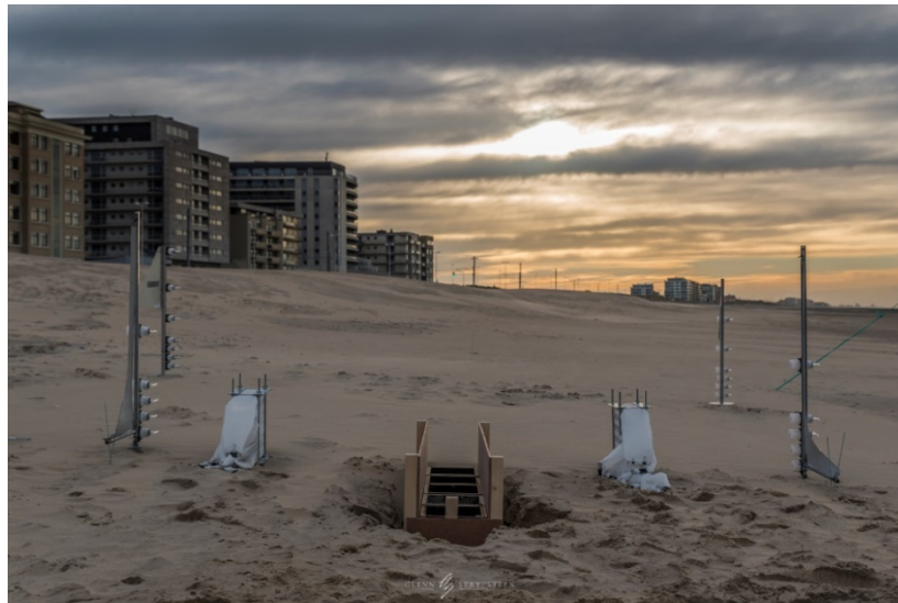
Part of the experimental set-up used on the beach of Mariakerke-Bad, November 21 st 2016. As seen in the figure, it consisted of fixed MWAC sand traps, rotatable MWAC sand traps, vertical traps and a horizontal trap.
