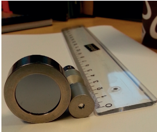
Figure 15. Dimensions of the RT12424 to the right compared to a standard size surface barrier detector for \alpha -spectrometry.
