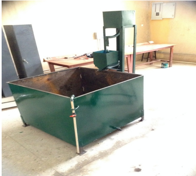
Plate 2 Full view showing the hopper, storage tank and the cage fish pond
