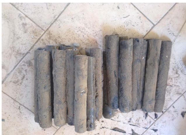
Fig. 1. Full culm bamboo coated with bitumen and sand.
