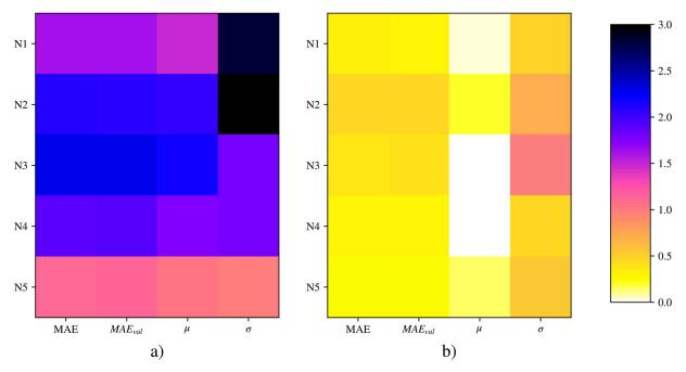
Fig 10. Heat graph for each layer of metrics (MAE, MAE on the test set, mean, and standard deviation) applied to the difference in prediction of actual data with respect to the model  $(Y - \hat{Y})$  for: a) Fourier model, b) TDNN model. The differences between predictions are shown in Celsius degrees.
