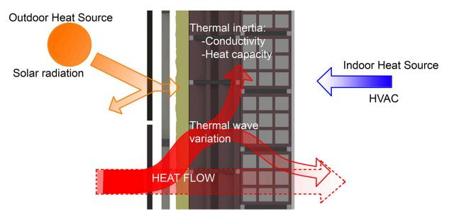
Fig 5. Diagram of the dynamic process of heat transmission through the enclosures.
