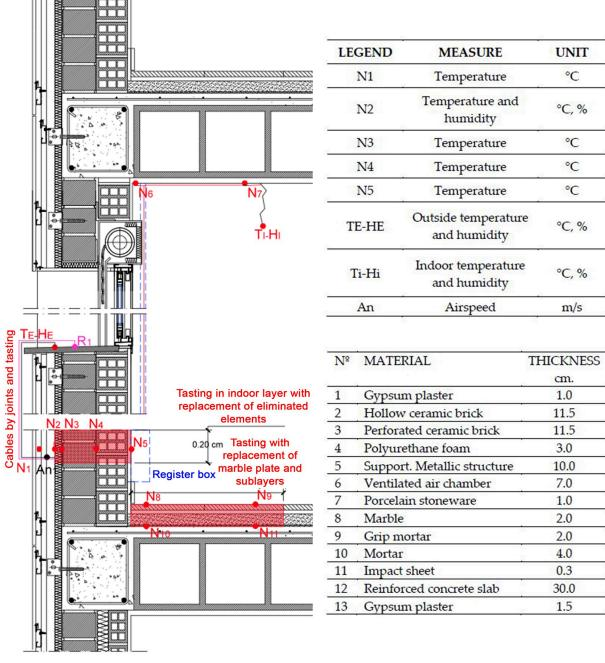
Fig 4. Chart of sensor location.
