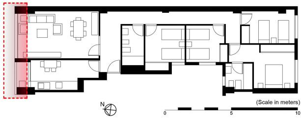
Fig 2. Floor plan of the type C dwelling. The red area represents the monitored ventilated facade.
