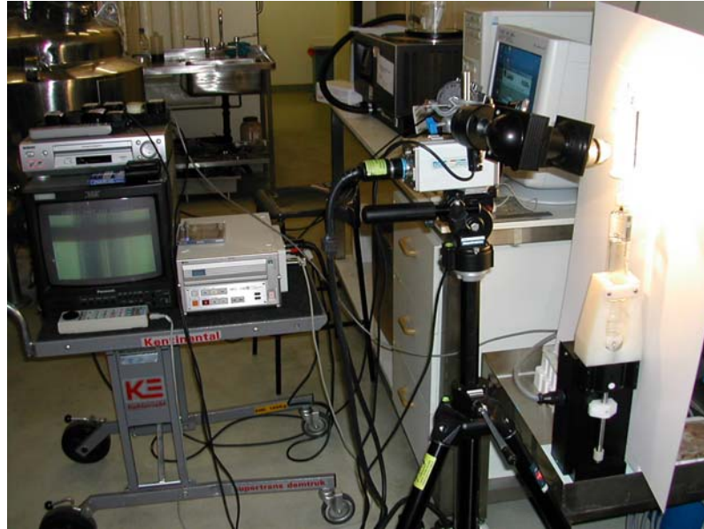
Figure 4.6 Experimental setup of the high-speed camera.
