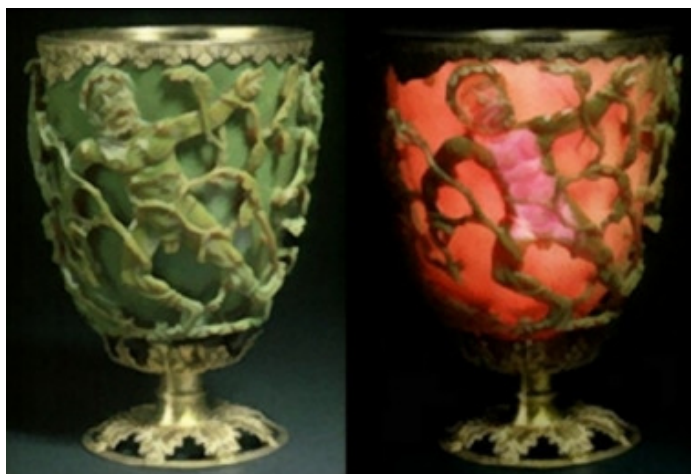
Figure 1-1 The Lycurgus cup, appears red in transmitted light (right) and green in reflected light (left) due to the presence of gold/silver colloids.
