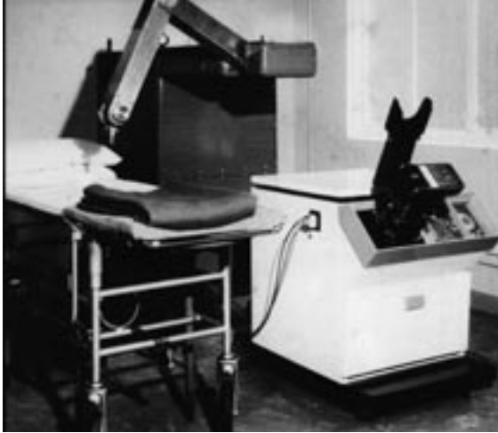
Figure 15: The world's first 'static' ultrasonic scanner using articulated arms. Professor Peter Wells wrote: 'This scanner, the precursor of the commercially manufactured machines which were in universal routine clinical use until the mid-1980s, when real-time scanners were introduced, was designed and constructed by Peter Wells at Bristol General Hospital in 1962–3. The electronics system was supplied by Nuclear Enterprises of Glasgow. The work was supported by a grant from the Medical Research Council.' Letter to Dr Daphne Christie, 5 January 2006.
