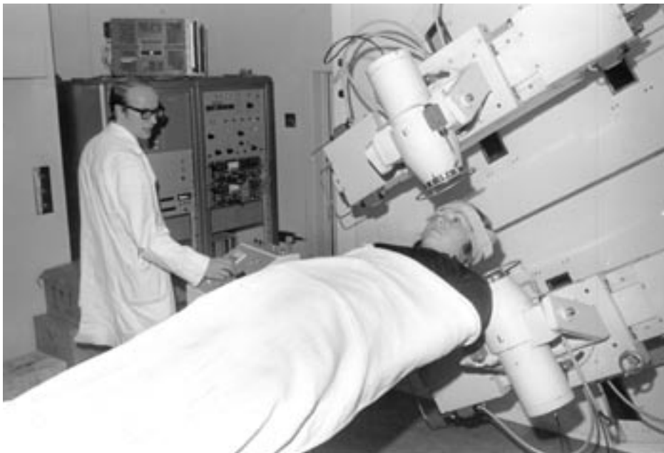
Figure 11: The first digital whole-body SPECT scanner (homemade). Dr Ian Keyes is operating the machine at the Royal Infirmary, Aberdeen, c. 1968.
