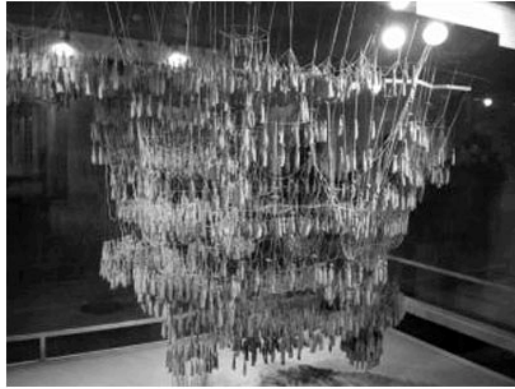
Figure 18 & 19: Gaudi's hanging model, a system of threads represents columns, arches, walls and vaults. Sachets with lead shot resemble the weight of small building parts ( http://me-wserver.mecheng.strath.ac.uk/group2003/group/Inspirational%20people/Antoni%20Gaudi_files/Antoni%20Gaudi.htm )
