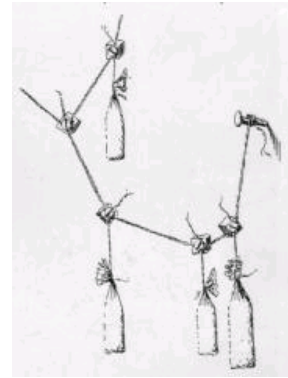
Figure 18 & 19: Gaudi's hanging model, a system of threads represents columns, arches, walls and vaults. Sachets with lead shot resemble the weight of small building parts ( http://me-wserver.mecheng.strath.ac.uk/group2003/group/Inspirational%20people/Antoni%20Gaudi_files/Antoni%20Gaudi.htm )
